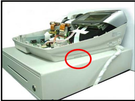
1. Cable entry location (Power supply unit cable entry position) (refer to 4-2 Block diagram Page 18 of the service manual)
