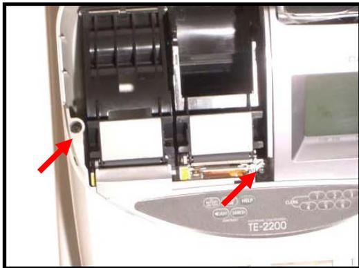
2. Remove the two screw. One on the left side of the receipt printer. The other on the right side of the Journal printer.
