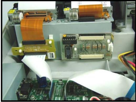
5. Replace the E272-PR PCB with FTP628MCL518 Adaptor PCB.
