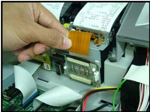
7. Push on the flexible cable from the top side.
